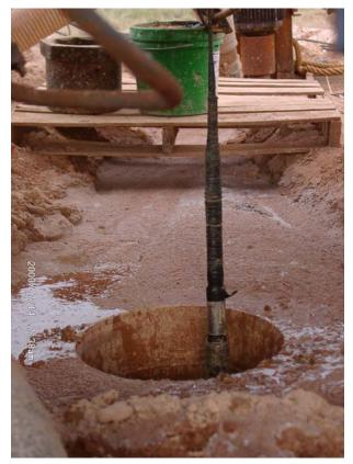
Logging tool at "zero depth" at initial logging of SNL-12.
